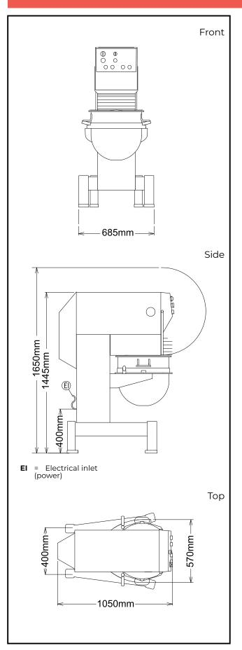
Electric 380-440 V/3N ph/50/60 Hz Supply voltage: Electrical power, max: 4 kW **Total Watts:** 4 kW Capacity: Performance (up to): 20 kg/Cycle 60 litres Capacity: Key Information: External dimensions, 685 mm Width: External dimensions, Depth: 1050 mm External dimensions, 1445 mm Height: **Shipping weight:** 306 kg ISO 9001; ISO 14001 kg **Cold water paste:** with Spiral hook
